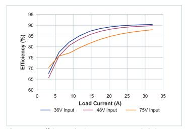
**Figure 12** — Efficiency vs. load at  $T_{CASE} = -40$ °C, nominal trim
