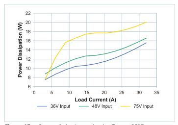
**Figure 15** — Power dissipation vs. load at  $T_{CASE} = 25$ °C, nominal trim
