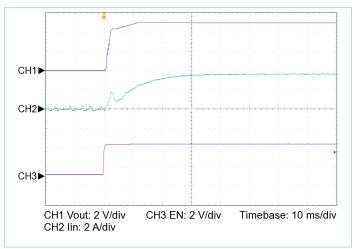
**Figure 20** — Start up from EN,  $V_{IN}$  = 48V,  $C_{OUT\_EXT}$  = 10000 $\mu$ F,  $R_{LOAD}$  = 0.156 $\Omega$
