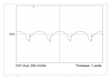
**Figure 22** — Output voltage ripple,  $V_{IN}$  = 48V,  $V_{OUT}$  = 5.0V,  $C_{OUT\_EXT}$  = 1000 $\mu$ F,  $R_{LOAD}$  = 0.156 $\Omega$
