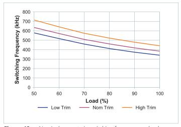
**Figure 19** — Nominal powertrain switching frequency vs. load, at nominal  $V_{\rm IN}$
