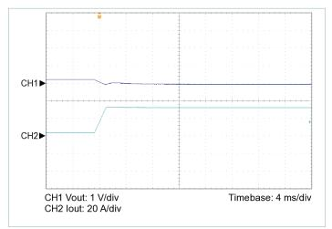
**Figure 8** — 10 – 100% load transient response,  $V_{IN}$  = 48V, nominal trim,  $C_{OUT\ EXT}$  = 1000 $\mu F$
