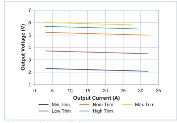
**Figure 6** — Ideal V<sub>OUT</sub> vs. load current, at 25°C case
