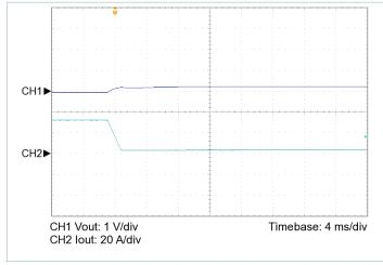
**Figure 7** — 100 – 10% load transient response,  $V_{IN}$  = 48V, nominal trim,  $C_{OUT\ EXT}$  = 1000 $\mu$ F
