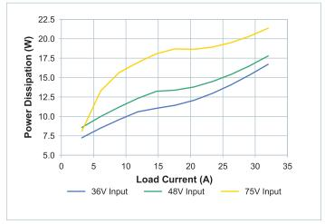
**Figure 17** — Power dissipation vs. load at  $T_{CASE} = 90$ °C, nominal trim
