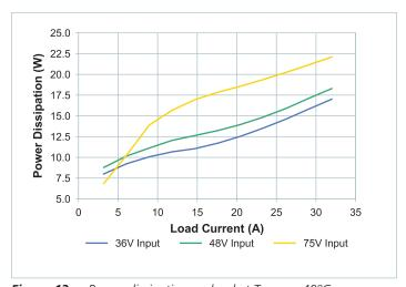
**Figure 13** — Power dissipation vs. load at  $T_{CASE} = -40$ °C, nominal trim
