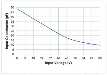
Figure 21 — Effective internal input capacitance vs. applied voltage
