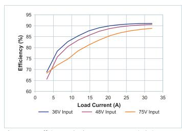
**Figure 14** — Efficiency vs. load at  $T_{CASE} = 25$ °C, nominal trim
