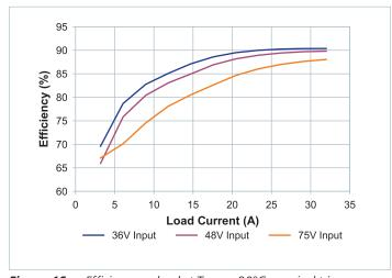
**Figure 16** — Efficiency vs. load at  $T_{CASE} = 90$ °C, nominal trim
