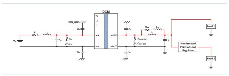
Typical application 2: single DCM3623x75H06A6yzz, to a non-isolated regulator, and direct to load
