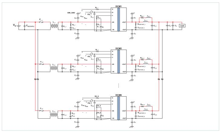
Figure 27 — DCM paralleling configuration circuit 2
