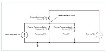
Figure 25 — One-side cooling thermal model
