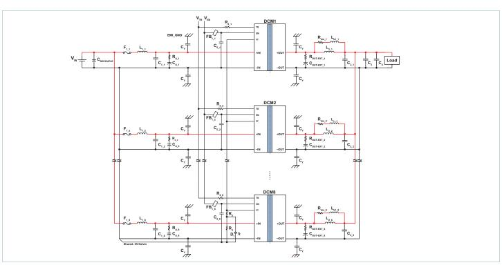
Figure 26 — DCM paralleling configuration circuit 1
