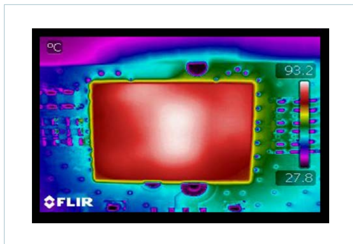
Figure 40 — Thermal image ( V_{IN} = 28V , I_{OUT} = 3.33A , CR, OLFM Evaluation PCB)
