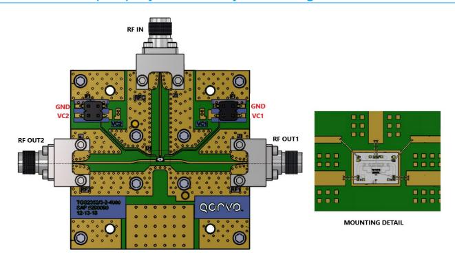
RF Layer is 0.010" thick Rogers Corp. RO4350B,  $\varepsilon r = 3.48$ . Metal layers are 0.5 oz. copper. The microstrip line at the connector interface is optimized for the Southwest Microwave end launch connector 1092-02A-5.
