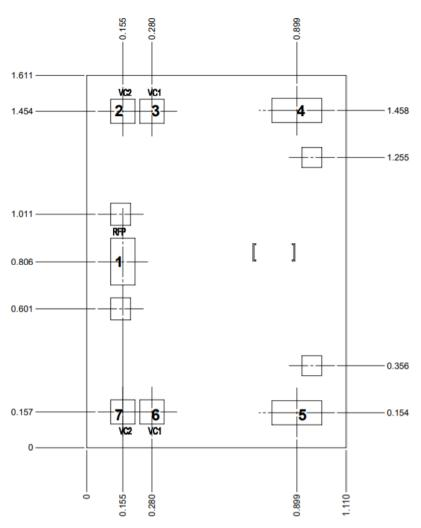
Unit: millimeters Thickness: 0.10 Die x, y size tolerance: +/- 0.050 Chip edge to bond pad dimensions is shown to center of pad
