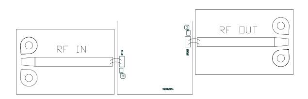
Note: RF Input and RF Output ports are not interchangeable.
