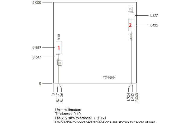
Chip edge to bond pad dimensions are shown to center of pad Ground is backside of die
