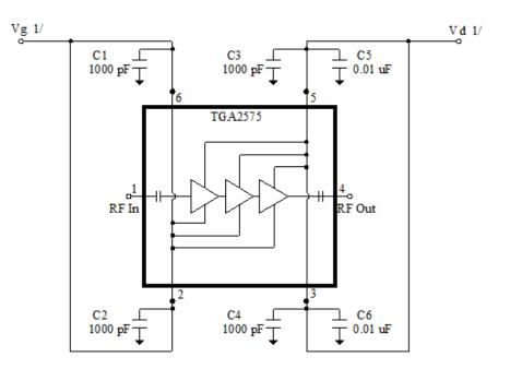
Vg must be biased from both sides (pins 2 and 6) Vd must be biased from both sides (pins 3 and 5)
