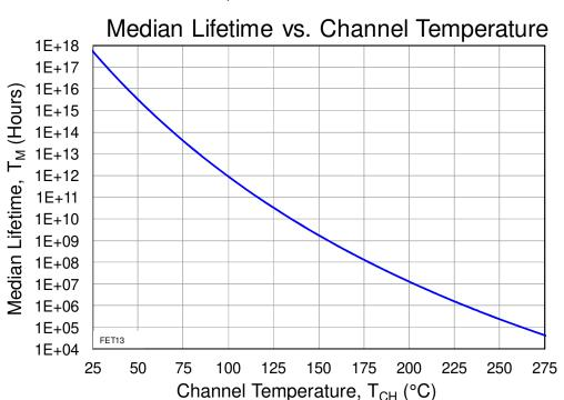
Test Conditions: 40 V; Failure Criteria = 10% reduction in  $I_{D MAX}$
